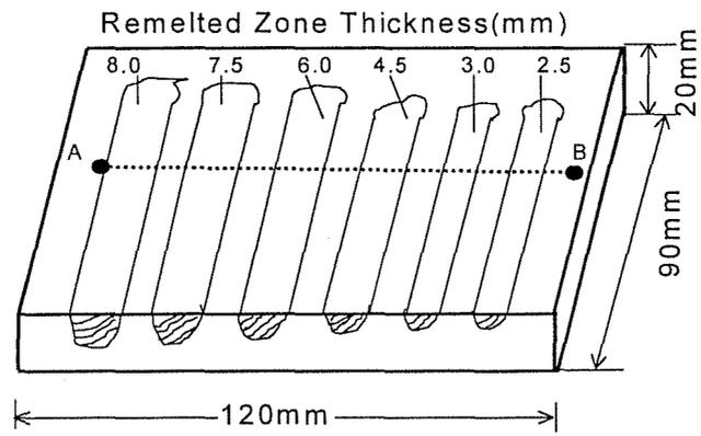
Fig.1 Schematic view of specimen for ultrasonic measurement.
