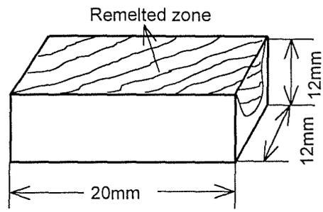
Fig.3 Test piece for measurement of density and velocity.
