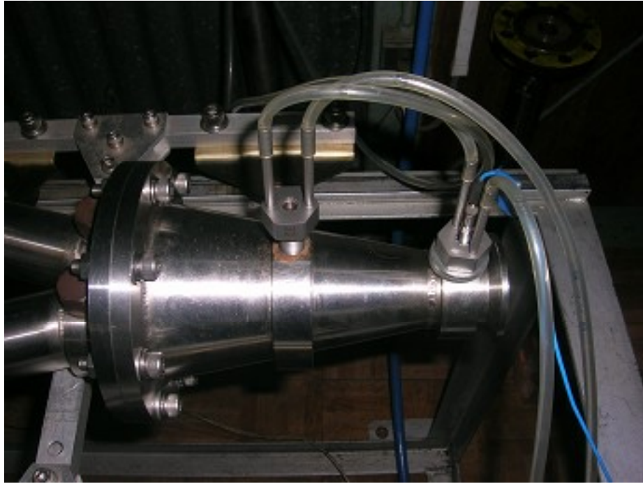
Fig.2.2.2 Photograph of water cool jacket adapter for pressure transducer
