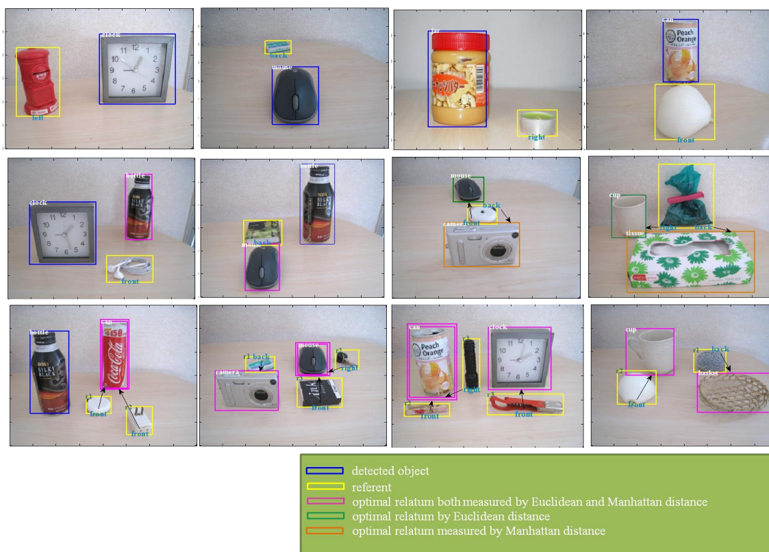
Fig.2. 13: Canonical spatial relation experiment result. Row 1: the scenarios of 1 referent vs. 1 relatum. Row 2: the scenarios of 1 referent vs. 1 or 2 relatum(s). Row 3: the scenarios of 2 or 3 referents vs. 2 relatums. The referent and chose relatum is linked by →
