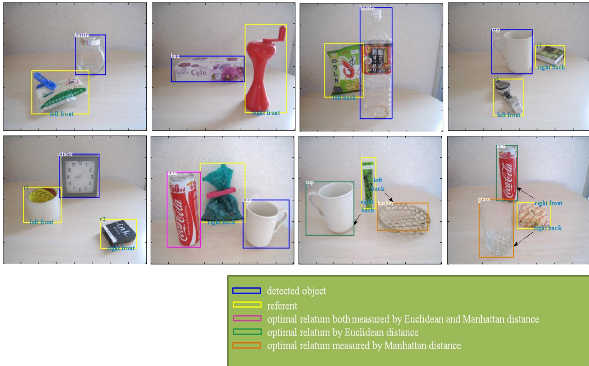
Fig.2. 14: Compound spatial relation experiment result. The referent and chose relatum is linked by →
