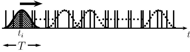
Figure 3.1: Transformation from a spike train to an instantaneous mean-firing-rate time series using a kernel function.
