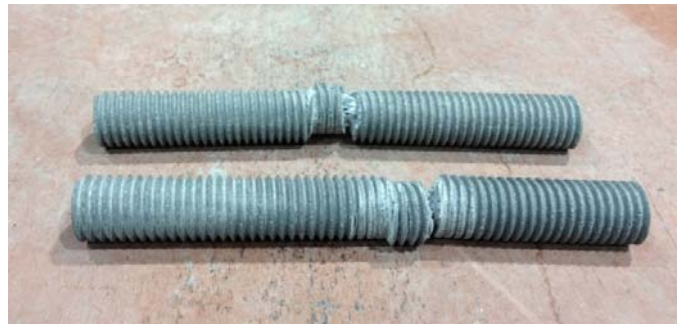
Fig. A7 Typical failure pattern of FRP bolt lap-shear test specimens (at 20°C, 60°C, and 90°C)
