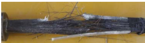
HFRP flange 70°C
