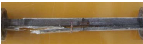
HFRP flange 30°C
