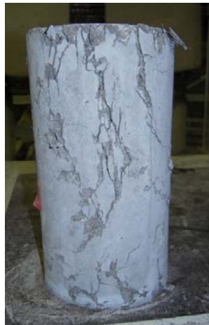
Fig. A4 Typical compression failure pattern of UFC cylinders (at all temperatures)
