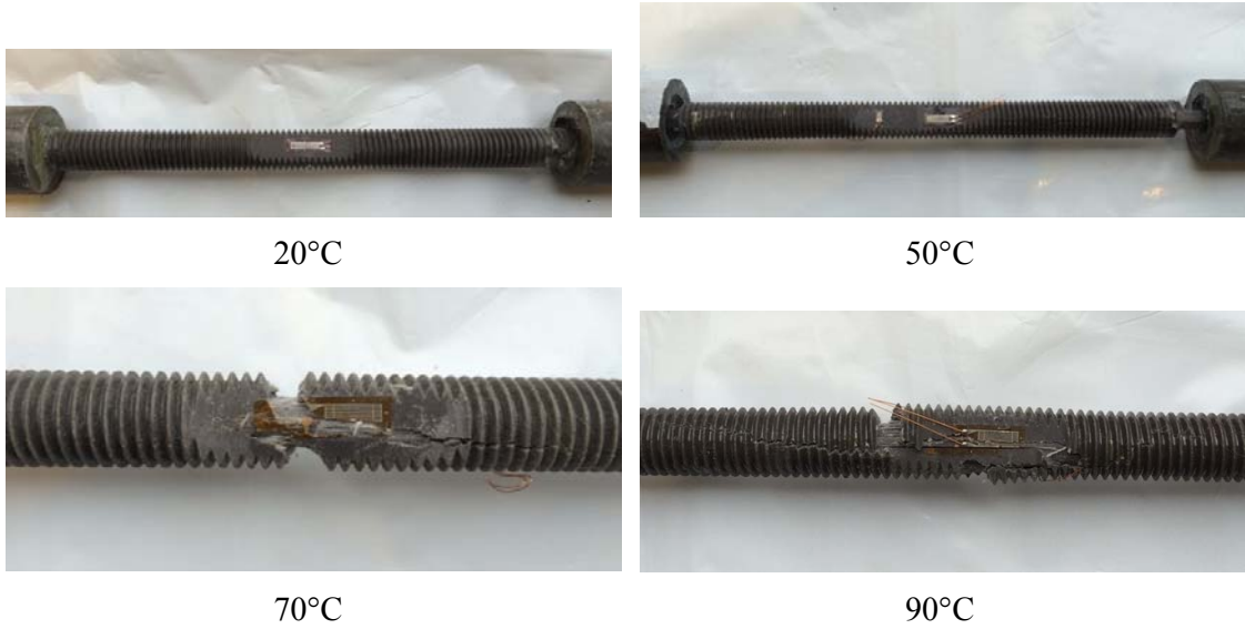
Fig. A5 Failure patterns of FRP bolt tensile test specimens
