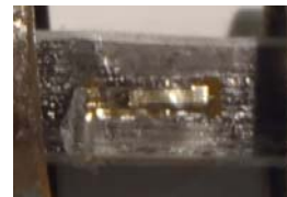
Kinking and crushing at 90°C
