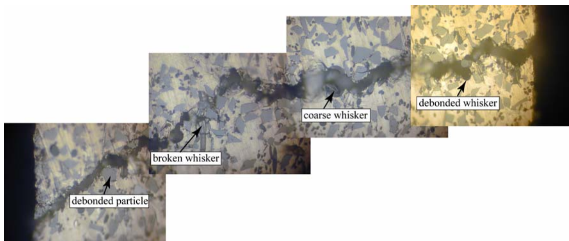
Fig.A2-2 Fracture path of homogeneous MMC ( \alpha = 0^\circ \sim 90^\circ ) under monotonic loading.
