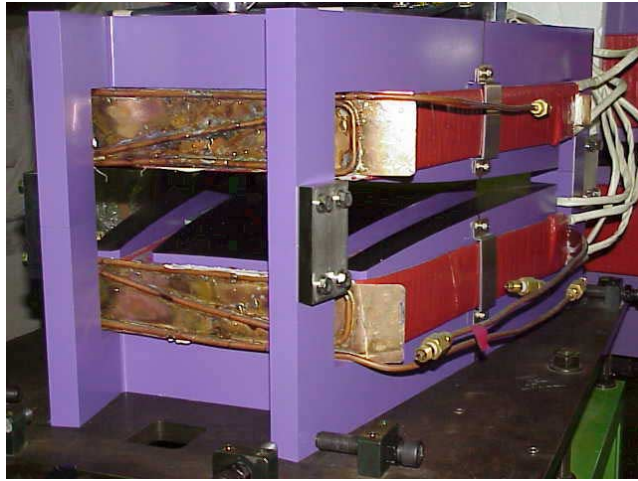
Figure 2.34: Prototype yoke free magnet
