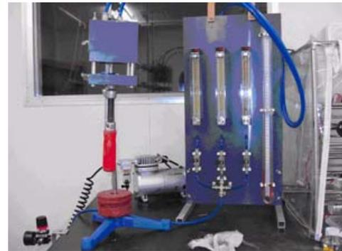
Fig. 2 Setup for the measurement of air permeability.
