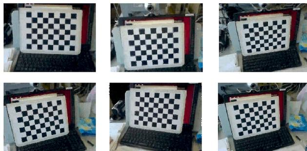
Fig.1. *Extracted calibration frames from an image stream by the implemented tool for handy camera calibration.*
