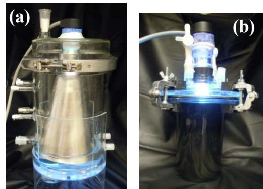
Fig. 2. Experimental setup for (a) gas-phase and (b) water-phase experiment with conical reflector.
