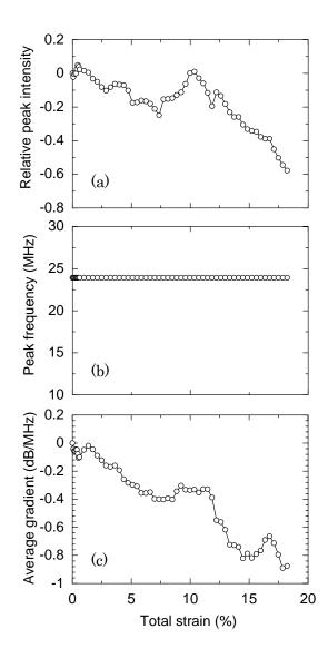
Fig.7 Change in ultrasonic parameters with total strain measured in real-time during tensile testing: (a) relative peak intensity, (b) peak frequency, (c) average gradient of transfer function.
