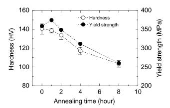
Fig.9 Change in Vickers hardness and yield strength with annealing time.
