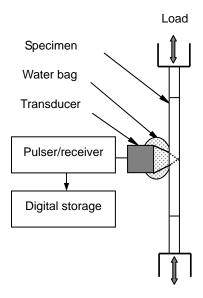
(b) Schematic representation of setup
