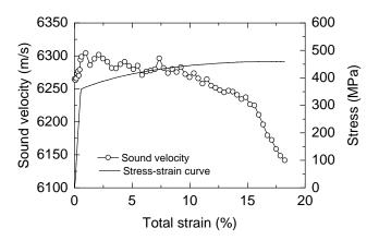
Fig.5 Typical stress-strain curve and change in sound velocity with total strain.
