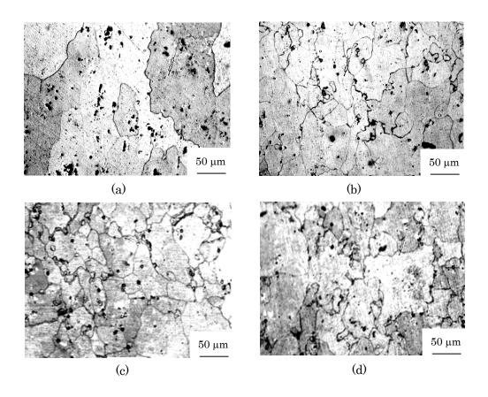
Fig.8 Optical micrographs: (a) before annealing; (b) annealing for  $2\,h$ ; (c) annealing for  $4\,h$ ; (d) annealing for  $8\,h$ . The rolling direction is vertical in the figure.
