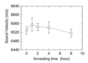
Fig.10 Change in sound velocity with annealing time.
