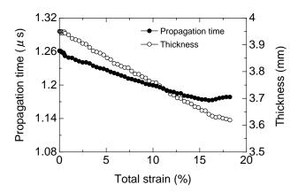
Fig.4 Change in propagation time and specimen thickness with total strain.
