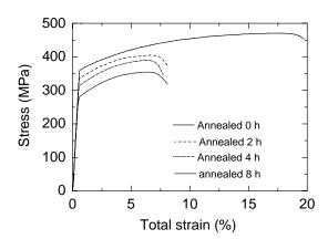
Fig.11 Typical stress-strain curves after annealing at 573 k for 0, 2, 4 and 8 hours.
