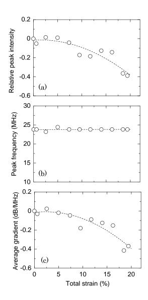
Fig.2 Change in ultrasonic parameters with total strain measured by conventional immersion method: (a) relative peak intensity; (b) peak frequency; (c) average gradient of transfer function.
