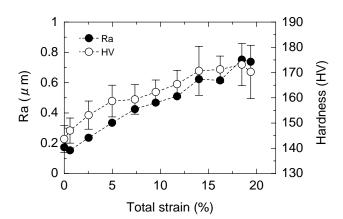
Fig.3 Change in surface roughness (Ra) and Vickers hardness (HV) with total strain.
