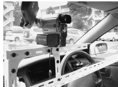
(a) Installation of camera B
