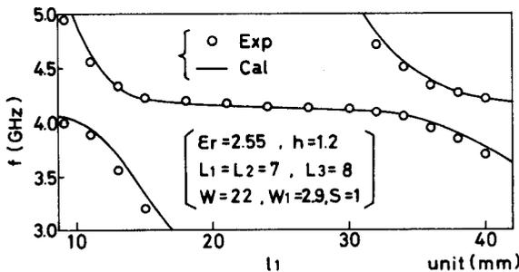
Fig. 4 Resonant frequencies versus open-circuited stub-length for test DB-MSA.
