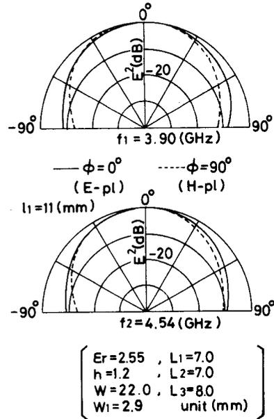
Fig. 5 Typical patterns for test DB-MSA.
