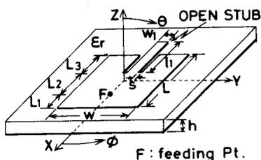
Fig. 1 Test DB-MSA and its coordinate system.
