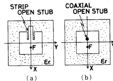
Fig. 2 Typical types of dual-band MSA
