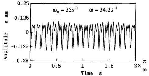
Fig. 6 Amplitude at the instance of rotational direction change
