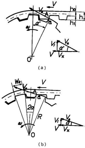
Fig. 1 Meshing collision of timing belt
