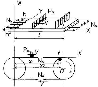
Fig. 3 Schematic of wide timing belt
