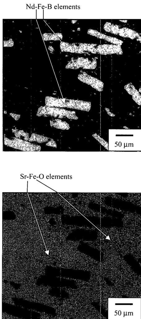
Fig. 9. Micrographs of the elements for  $\text{Nd}_2\text{Fe}_{14}\text{B}$  and  $\text{SrO}\cdot 6\text{Fe}_2\text{O}_3$  measured by EPMA for specimen C.
