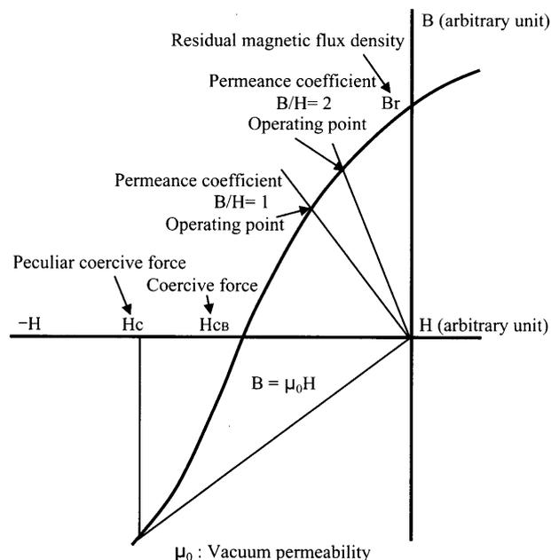
Fig. 4. Description of general technical terms concerning the demagnetization curve of the  $B$ - $H$  curve.
