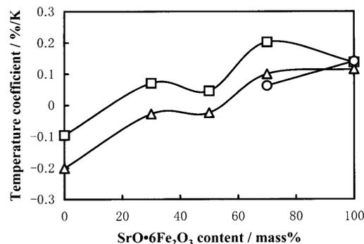
Fig. 8. Effect of  $\text{SrO}\cdot 6\text{Fe}_2\text{O}_3$  addition on the temperature coefficient of coercive force  $H_{cB}$  for a  $\text{Nd}_2\text{Fe}_{14}\text{B}$  magnet.
