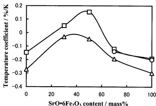
Fig. 5. Effect of  $\text{SrO}\cdot 6\text{Fe}_2\text{O}_3$  addition on the temperature coefficient of residual magnetic flux density  $B_r$  for a  $\text{Nd}_2\text{Fe}_{14}\text{B}$  magnet.  $\square$  297-323 K,  $\triangle$  323-373 K,  $\circ$  373-413 K.
