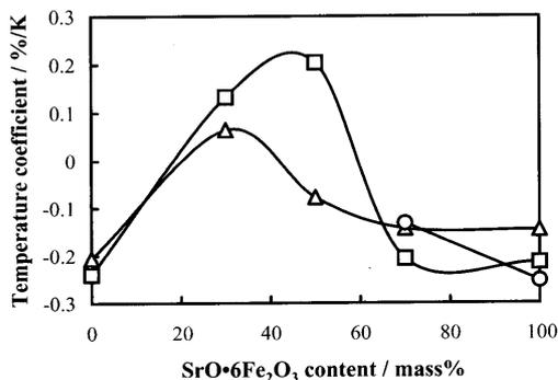
Fig. 7. Effect of  $\text{SrO}\cdot 6\text{Fe}_2\text{O}_3$  addition on the temperature coefficient of magnetic flux density at operating point of permeance coefficient  $P_c(B/H) = 2$  for a  $\text{Nd}_2\text{Fe}_{14}\text{B}$  magnet.
