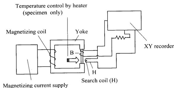
**Fig. 1.** Automatic equipment for measuring hysteresis loop by DC drive.
