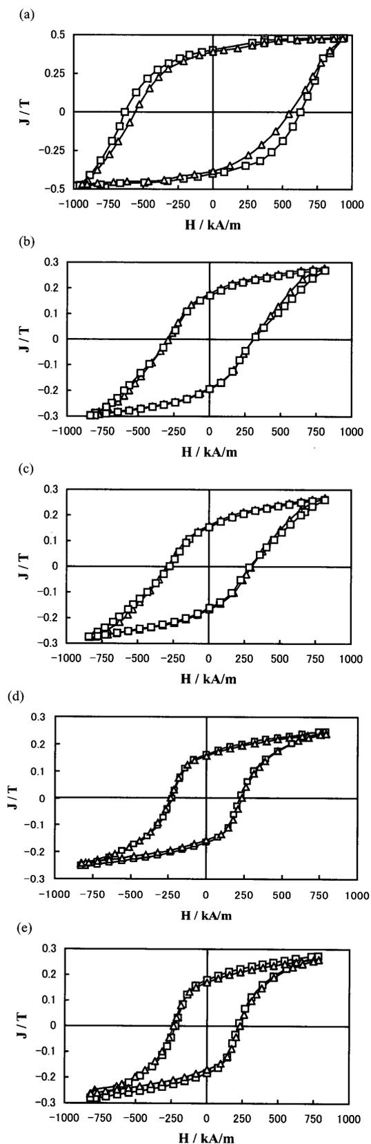
Fig. 3.  $J$ - $H$  loops of composite  $\text{Nd}_2\text{Fe}_{14}\text{B}$ - $\text{SrO}\cdot 6\text{Fe}_2\text{O}_3$  magnets.  $\square$  297-323 K,  $\triangle$  323-373 K.
