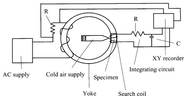
**Fig. 2.** System for hysteresis loop measurement by a pulse magnetization measuring device incorporating a superconductor for the generation of large current.
