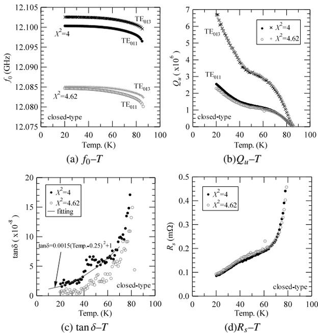
**Fig. 10** Measured results of closed-type resonators for  $X^2=4$  and 4.62.
