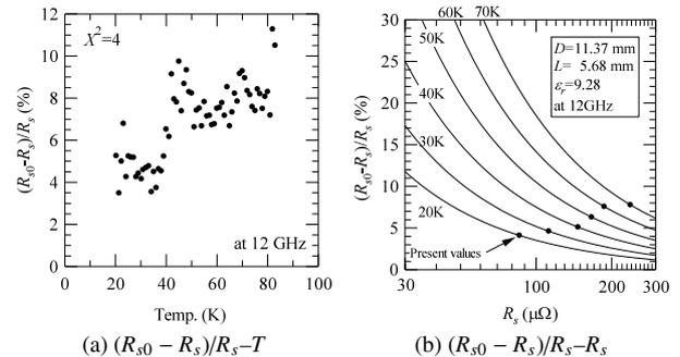
**Fig. 11** Calculated errors of  $R_s$  at 12 GHz when  $\tan \delta = 0$ .
