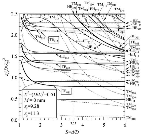
(b) For TE<sub>013</sub> mode resonator.
