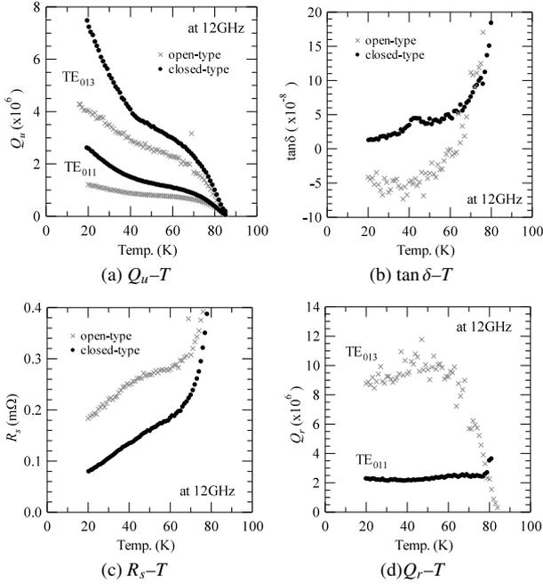
**Fig. 9** Measured results of open-type and closed-type resonators for  $X^2=4$ .
