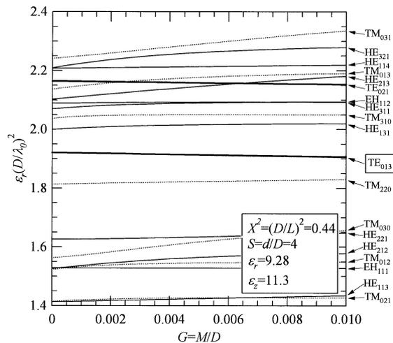
(b) For TE<sub>013</sub> mode resonator.
