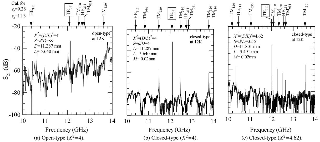
**Fig. 8** Measured frequency responses for TE<sub>011</sub> resonators at 12 K.
