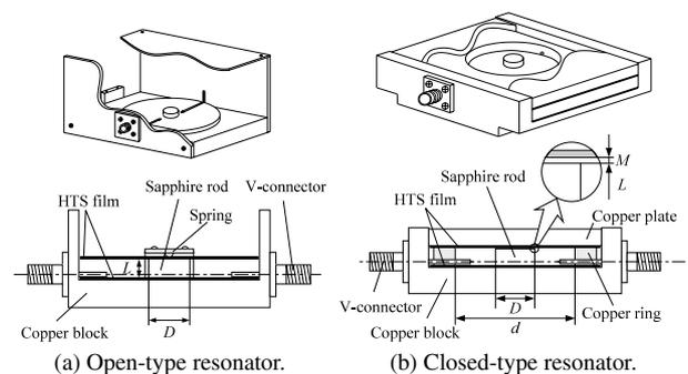
**Fig. 1** Sapphire rod resonator structures of two types.
