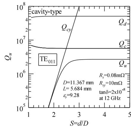
**Fig. 5** Calculated results of  $Q$  values for the  $TE_{011}$  mode cavity-type resonator.
