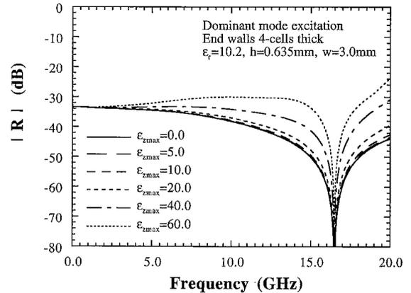
Fig. 2 Performance of the end walls with varying values of  $\epsilon_{zmax}$ . The MPML end walls are 4-cells thick with an assigned  $R_{th} = 10^{-3}$  ( $-60$  dB). The dominant mode of the microstrip line is excited.
