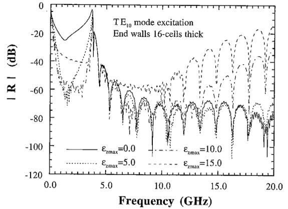
**Fig. 8** Performance of the MPML end walls in a rectangular waveguide. The MPML end walls are 16-cells thick with an assigned  $R_{th}=10^{-4}$  (-80 dB).  $TE_{10}$  mode of the waveguide is excited.
