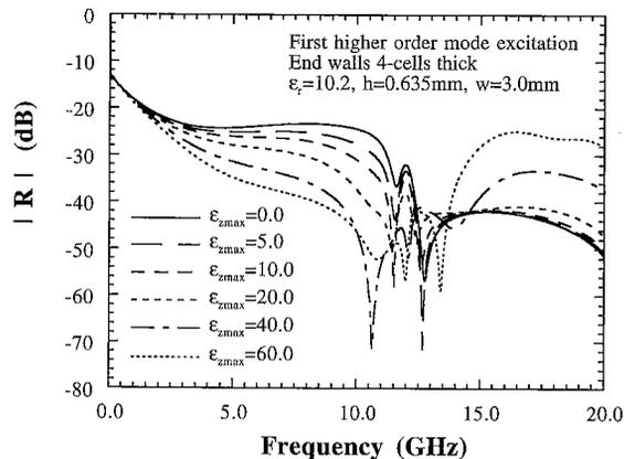
**Fig. 4** Performance of the end walls with varying values of  $\epsilon_{zmax}$ . The MPML end walls are 4-cells thick with an assigned  $R_{th}=10^{-3}$  ( $-60$  dB). The first higher order mode of the microstrip line is excited.
