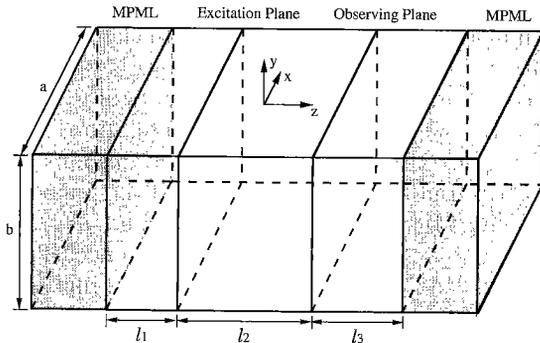
**Fig. 7** A rectangular waveguide terminated by two MPML end walls.
