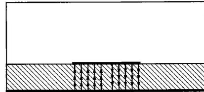
Fig. 3 Excitation of the first higher order mode of the microstrip line by the vertical electric field imposed in an asymmetrical fashion in the excitation plane underneath the metal strip.
