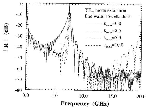
**Fig. 9** Performance of the MPML end walls in a rectangular waveguide. The MPML end walls are 16-cells thick with an assigned  $R_{th}=10^{-4}$  (-80 dB).  $TE_{20}$  mode of the waveguide is excited.
