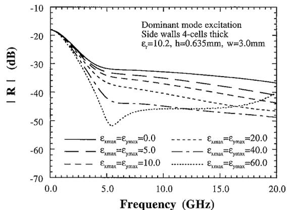
**Fig. 5** Performance of the side walls with varying values of  $\epsilon_{xmax}$  and  $\epsilon_{ymax}$ . The MPML side walls are 4-cells thick with an assigned  $R_{th}=10^{-3}$  ( $-60$  dB). The dominant mode of the microstrip line is excited.
