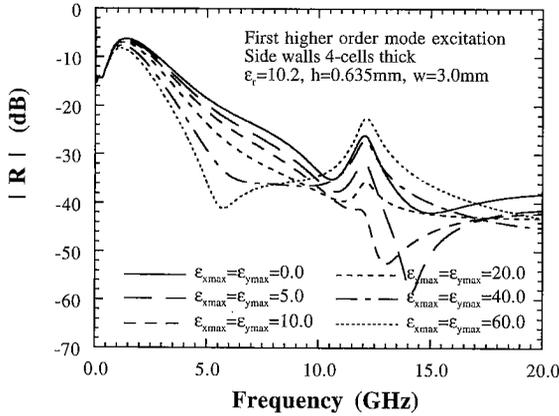
**Fig. 6** Performance of the side walls with varying values of  $\epsilon_{xmax}$  and  $\epsilon_{ymax}$ . The MPML side walls are 4-cells thick with an assigned  $R_{th}=10^{-3}$  (-60 dB). The first higher order mode of the microstrip line is excited.
