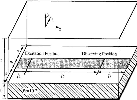
Fig. 1 A microstrip line terminated by MPML boundaries.
