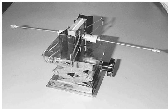
**Fig. 5** A photograph of the stripline resonator illustrated in Fig. 4.
