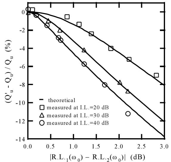
**Fig. 6** Comparison of the measured and predicted errors between  $Q'_u$  and  $Q_u$  by the insertion loss and return loss method, respectively.
