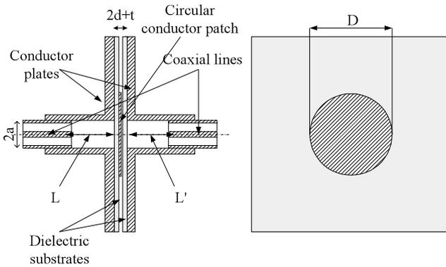
**Fig. 4** Configuration of a stripline circular patch resonator operating at  $TM_{010}$  mode.
