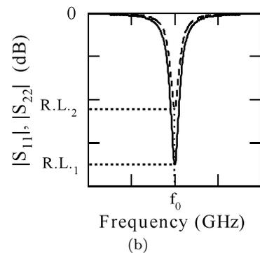
Fig. 2 (a) Transmission coefficient of a resonator, with the resonant frequency  $f_0$  and the 3-dB frequencies  $f_1$  and  $f_2$ . (b) Reflection coefficients with the return losses  $R.L._1$  and  $R.L._2$  at the resonant frequency  $f_0$ .
