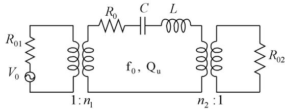
Fig. 1 Equivalent circuit of a transmission-type resonator.
