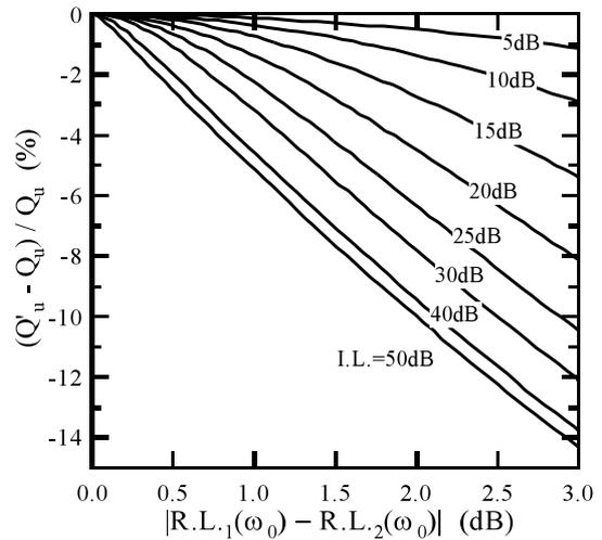
**Fig. 3** The calculated error between  $Q'_u$  and  $Q_u$  versus  $|R.L._1(\omega_0) - R.L._2(\omega_0)|$ . The insertion loss  $I.L.(\omega_0)$  is varied from 5 dB to 50 dB.
