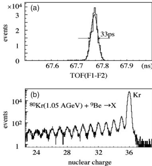
FIG. 2. (a) TOF spectrum between the scintillators at F1 and at F2. A Gaussian fit for the peak gives the time resolution of 33 ps (FWHM). (b) Nuclear charge spectrum of fragments from  $^{80}\text{Kr}$  fragmentation at 1.05 A GeV, measured in an ionization chamber. The primary beam with  $Z = 36$  was used for calibration.
