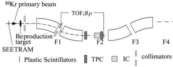
FIG. 1. Experimental setup at the fragment separator FRS
