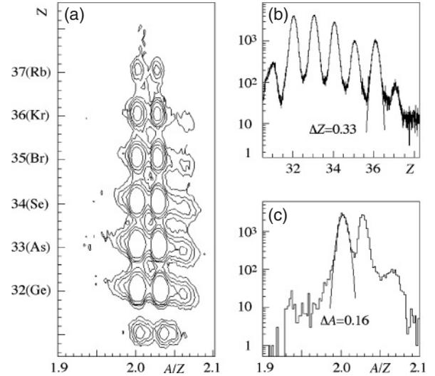
FIG. 3. (a) Two-dimensional contour plot of  $Z$  versus  $A/Z$  for the FRS setting selecting  $^{72}\text{Kr}$  as the central fragment. (b)  $Z$  projection of Fig. 3(a). The solid line indicates a Gaussian fit to the  $Z = 36$  peak, yielding a  $\Delta Z = 0.33$ . (c)  $A/Z$  projection spectrum for the  $Z = 36.0 \pm 0.28$  slice of Fig. 3(a). The solid line indicates a Gaussian fit to the  $^{72}\text{Kr}$  peak, yielding  $\Delta A = 0.16$ .
