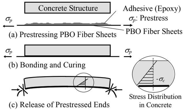
Figure 4. Strengthening of concrete structure with prestressed PBO fiber sheets
