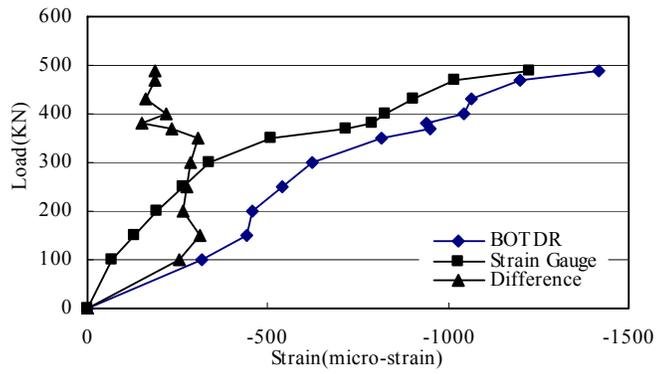
Figure 21. Compressive strain measurement of concrete compared with strain gauges in middle span.
