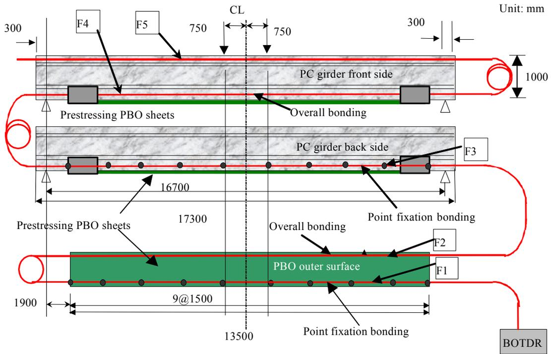
Figure 11. Fiber optic sensor installed on the strengthened PC girder with different bonding methods.
