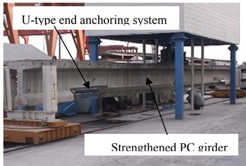
Figure8. The PC specimen strengthened with P-PUT method
