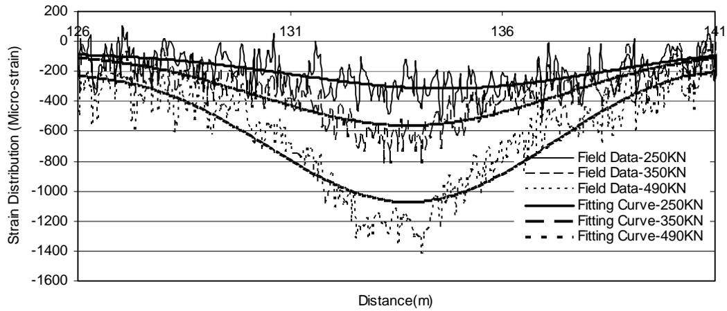
Figure 19. Compression strain measurement along the compression concrete flange.
