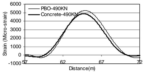
(a) Strain distribution under 490 KN
