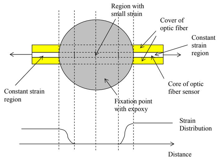
Figure 15. Strain distribution on the fixation point.
