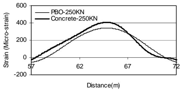
(a) Strain distribution under 250 KN
