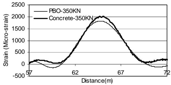
(b) Strain distribution under 350 KN
