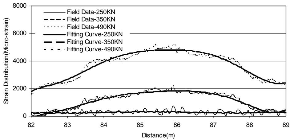
(b) Strain distribution along tension concrete flange
