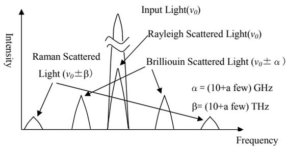
Figure 1 Scattered light spectrum in an optic fiber.
