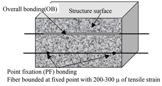
Figure 9. Installation methods of optical fiber sensors.
