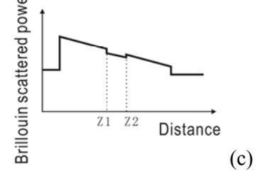
Figure 2 Brillouin back-scattering distribution at difference frequencies along the optic fiber.
