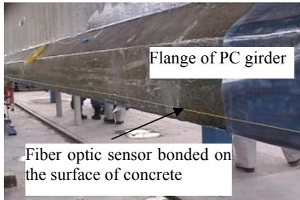
(a) Fiber optic sensor bonded on the surface of concrete
