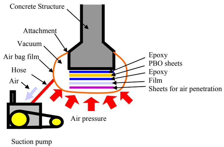
Figure 6. Air bag system for PBO bonding.
