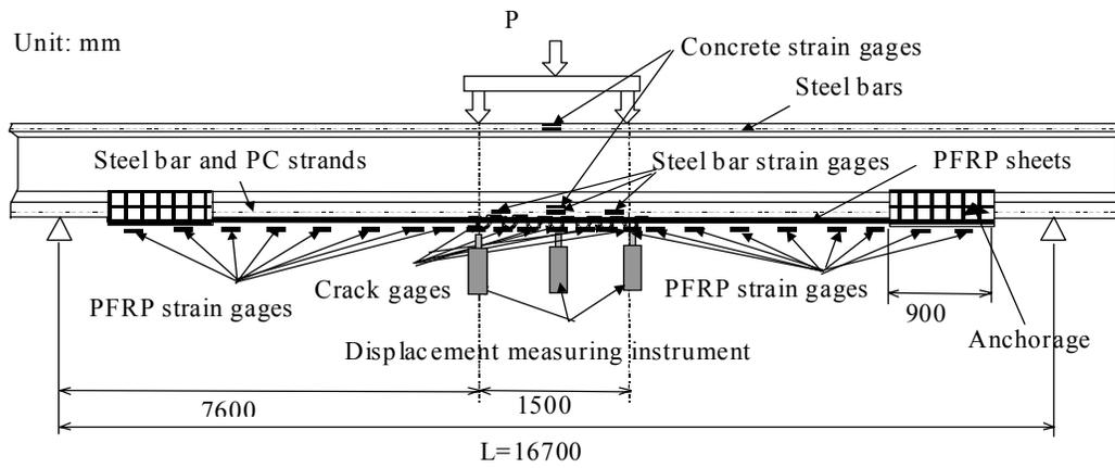
Figure 3. Test set up of the four point bending experiment of the PC girder strengthened by prestressed PBO sheets.
