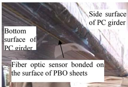
(b) Fiber optic sensor bonded on the surface of PBO sheets
