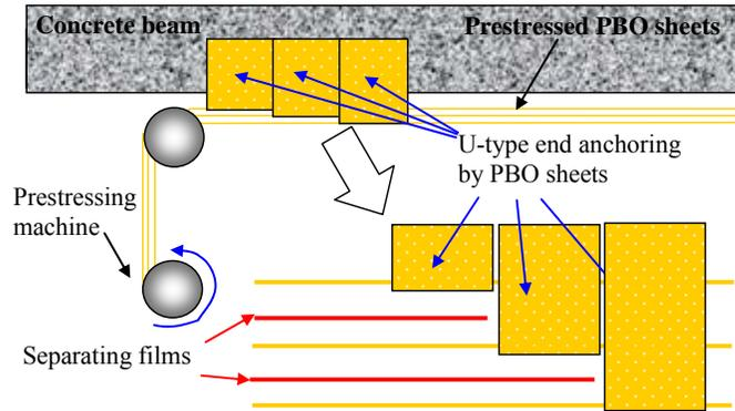
Figure 7. U-type end anchoring system by bonded PBO sheets
