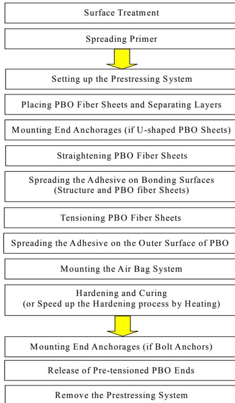
Figure 5. Flowchart of P-PUT strengthening method.
