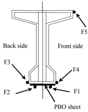
Figure 10. Installation position of fiber optic sensor on the cross section of strengthened PC girder.
