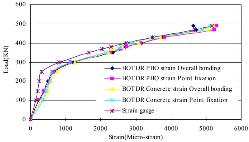
Figure 20. Tension strain measurement of PBO sheets compared with strain gauges in middle span.
