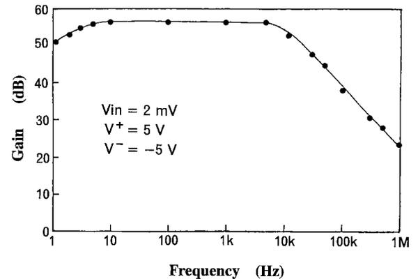
Fig. 9 Total frequency response of amplifier.
