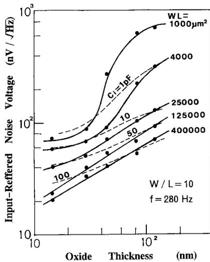
Fig. 5 Experimentally observed input-referred noise voltage of PMOSFETs having different gate areas and a same channel ratio ( $W/L$ ).
