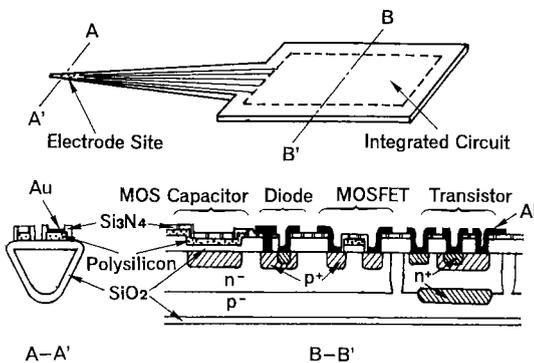
Fig. 1 Structure of integrated electrode probe.
