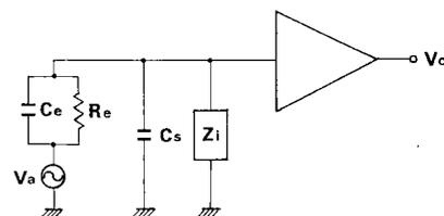
Fig. 3 Equivalent circuit of microelectrode and amplifier.
