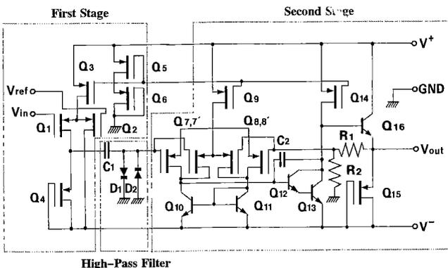
**Fig. 4** Design of Bi-MOSFET amplifier for microelectrode.
