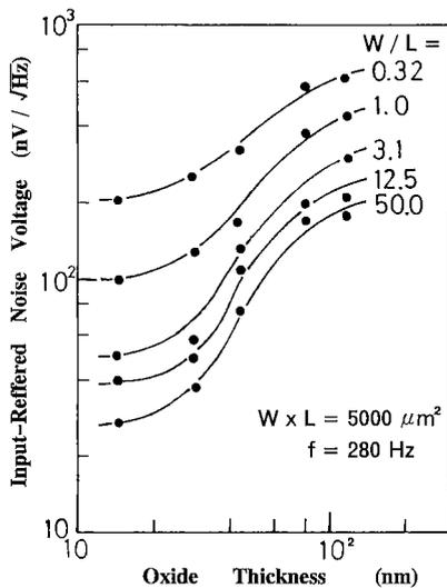
Fig. 6 Experimentally observed input-referred noise voltage of PMOSFETs having different channel ratios ( $W/L$ ) and a same gate area.
