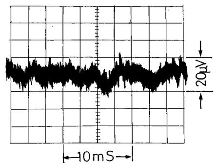
Fig. 10 Noise voltage waveform of amplifier.
