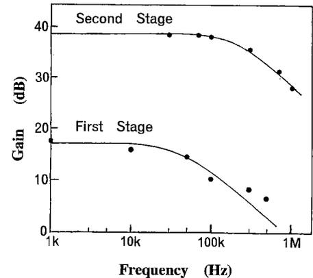
Fig. 8 Frequency responses of the first and the second stages in the amplifier.
