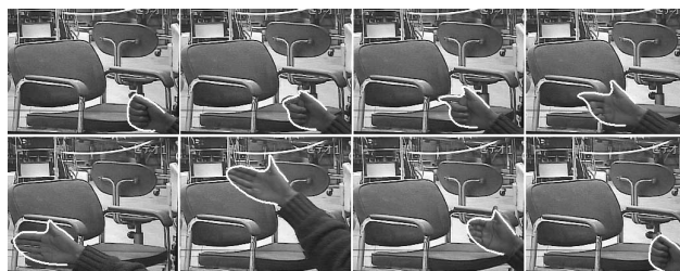
Fig. 8 Tracking by model B . A test sequence with the complicated background was given, the tracker of model B successfully tracked the hand gesture with the rapid changes in shapes and positions. From left-top to right-down, the frame numbers are 1,21,25,31,46,77,92 and 105, respectively.
