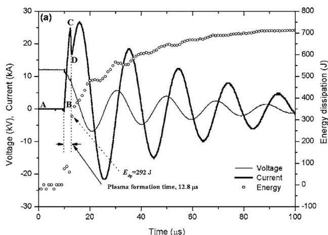
FIG. 1. Copy of Fig. 2(a) from Ref. 1. Letters are inserted to indicate the stages of the discharge.
