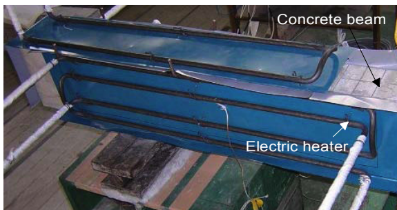
Fig. 16 Concrete beam with electric heaters.
