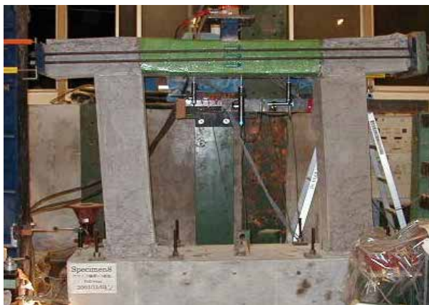
b) Failure of specimen S-4
