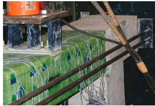
d) Strain measuring of beam of specimen S-4
