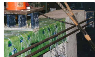
a) Strengthened beam (fully wrapped with AFRP)
