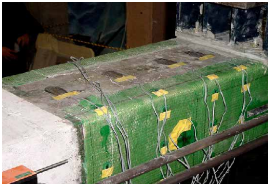
c) Strain measuring of beam of specimen S-3
