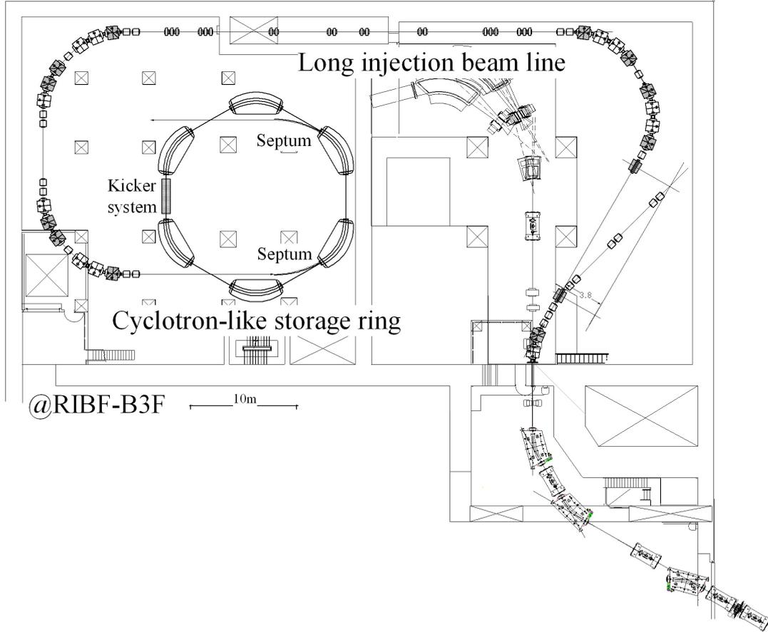
Fig. 1. Floor arrangement of our apparatus, presently under design.
