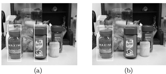
Fig. 15 (a) Detected object along with false positive (b) No result of false positive after inclusion of the previous false positive image in the negative training set.
