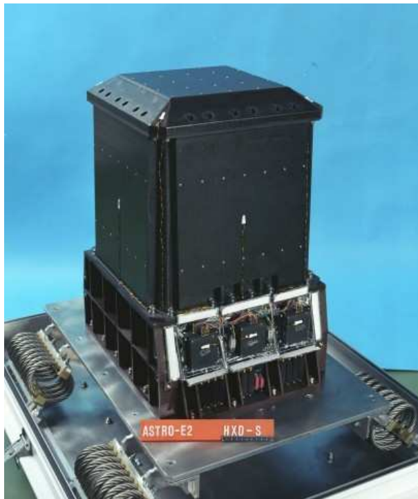
Fig. 1. Hard X-ray Detector before installation.
