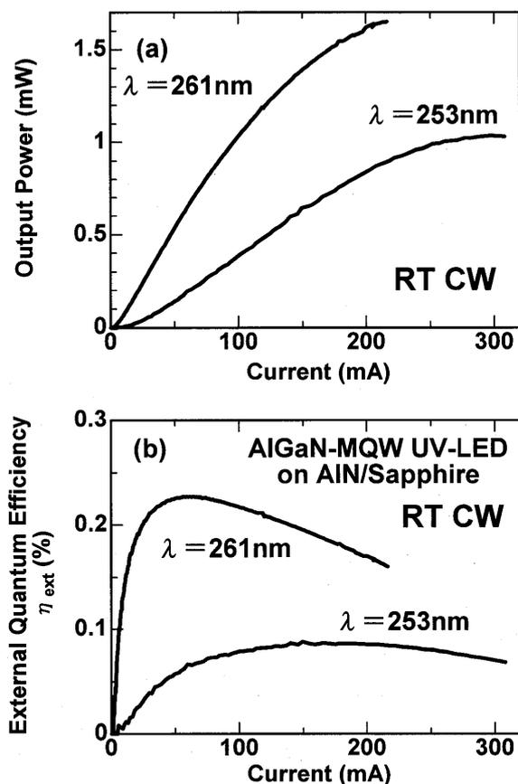
Figure 6 (a) output power and (b) external quantum efficiency (EQE)  $\eta_{\text{ext}}$  for 253 nm and 261 nm AlGaIn-MQW LEDs as a function of current measured under RT CW operation
