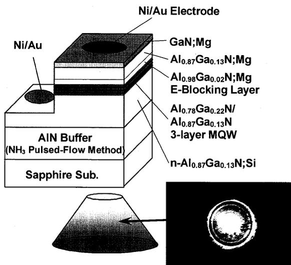
Figure 4 Schematic of the sample structure of an AlGa<sub>N</sub> MQW deep-UV LED with emission wavelength of 227.5 nm fabricated on a ML-AlN buffer and an emission pattern image observed from back side of sapphire substrate
