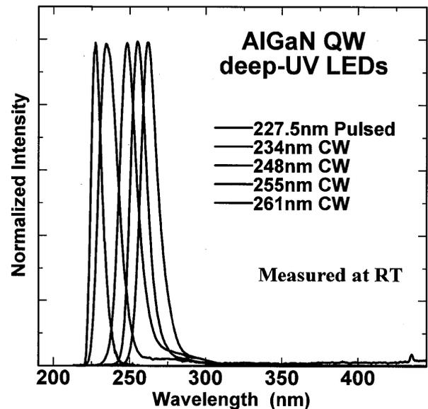
Figure 5 Electroluminescence (EL) spectra of the fabricated AlGa<sub>N</sub>-MQW LEDs with wavelengths of 227.5 nm under pulsed operation and 234, 248, 255 and 261 nm under CW operations, all measured at room temperature (RT), with injection current of 30-50 mA
