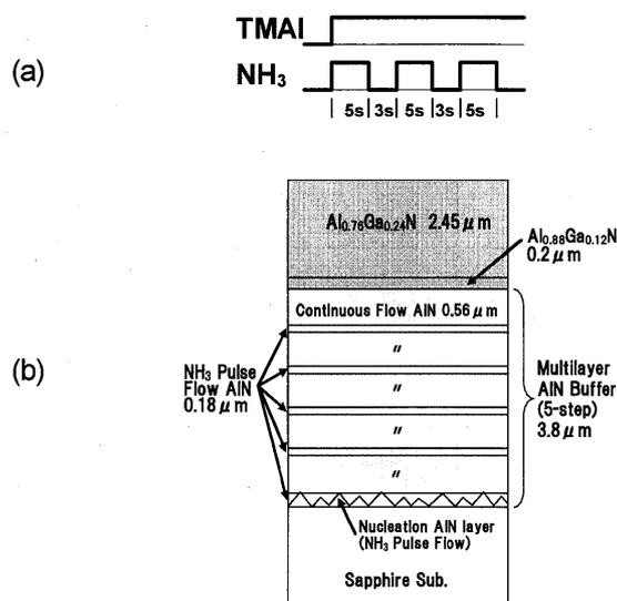
Figure 1 (a) Gas flow sequence used in  $\text{NH}_3$  pulse-flow growth
