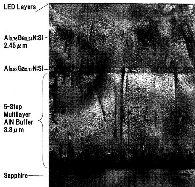
Figure 2 Cross-sectional TEM image of an AlGaN-MQW UV LED with emission wavelength of 253 nm
