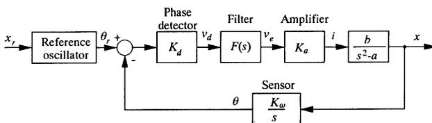
Fig. 2 Block diagram of PLMS using a linearized model in case of one-sided operation
