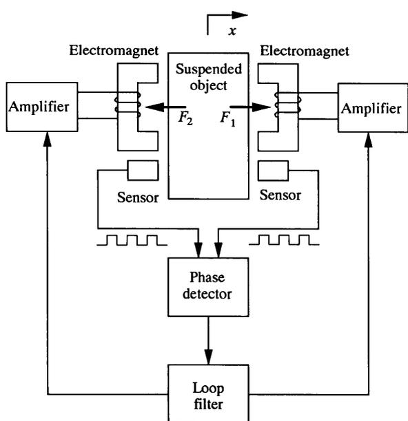
Fig. 3 Schematic diagram of PLMS in case of differential operation
