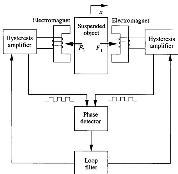
Fig. 6 Self-sensing configuration of PLMS
