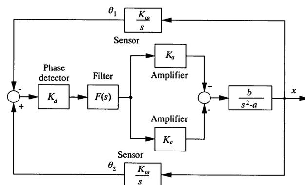
Fig. 4 Block diagram of PLMS using a linearized model in case of differential operation
