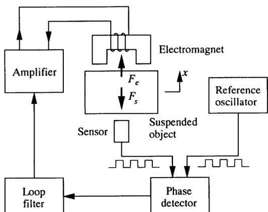
Fig. 1 Schematic diagram of PLMS in case of one-sided operation
