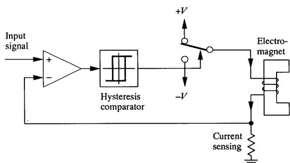
Fig. 5 Schematic diagram of hysteresis amplifier
