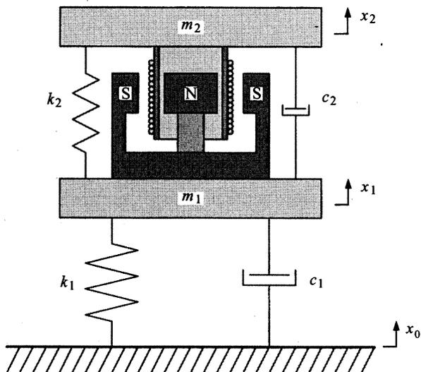
Fig. 5 Basic model of a zero-compliance system
