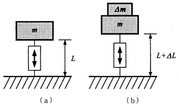
Fig. 3 Negative stiffness for direct disturbances
