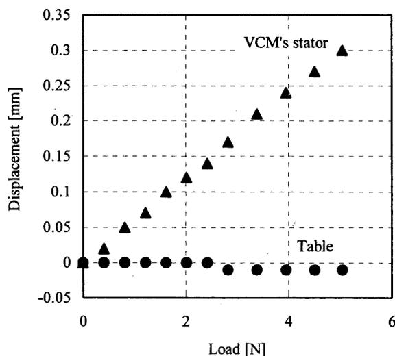
Fig. 8 Displacements of the VCM's stator and the table when load force acts on the table
