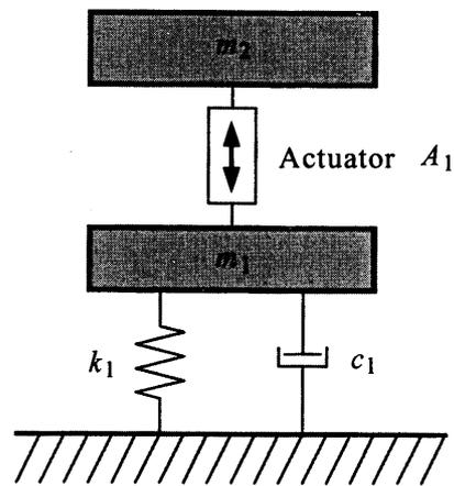
Fig. 2 Structure of vibration isolation system
