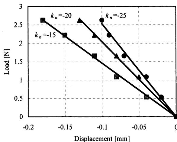
Fig. 7 Relation between the displacement of the table and load acting on the table
