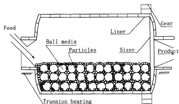
Fig. 1 Vertical section through a ball mill
