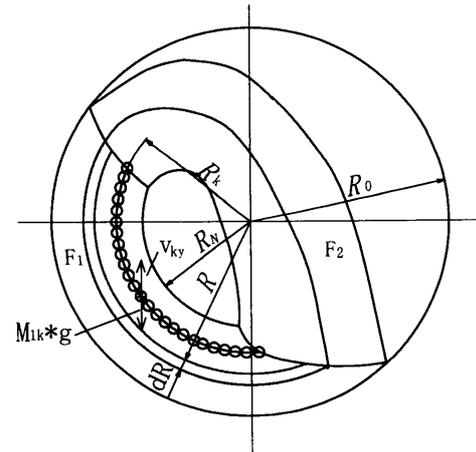
Fig. 6 Charge analysis of tumbling ball mill
