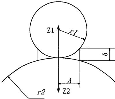
Fig. 4 Contact analysis of collision
