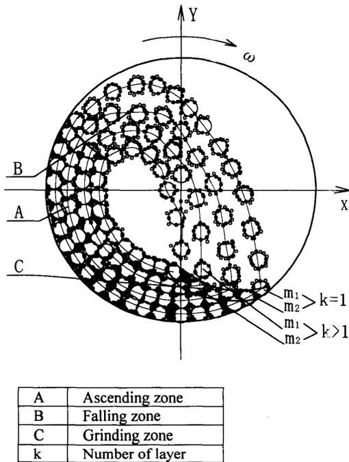
Fig. 2 Cross section of tumbling ball mill
