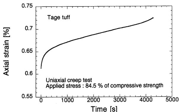
Fig. 4. Creep curve of Taya tuff. Uniaxial creep test. Courtesy of Dr. Yamabe of Saitama Univ.
