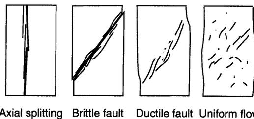
Fig.3. Sketch of macroscopic failure mode in triaxial compression tests by Donath et al. [11]. Failure modes corresponds to the legends in Fig. 2 .
