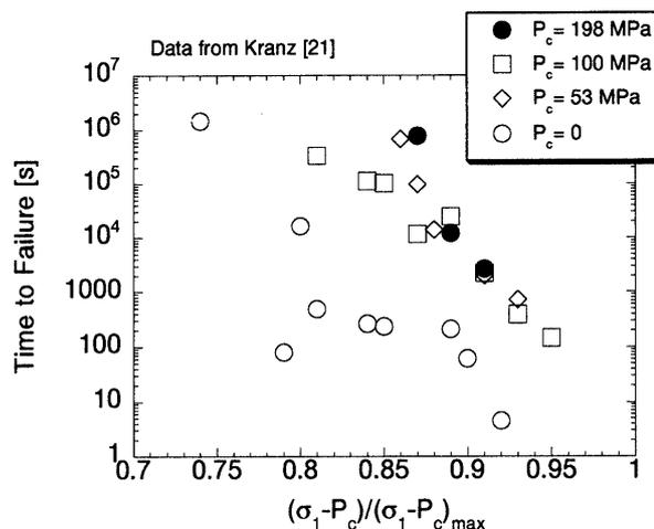
Fig. 5. Effect of confining pressure  $p_c$  and stress difference  $(\sigma_1 - p_c)$  on time to fracture in creep tests of Barre granite. ( $\sigma_1$ : maximum compressive stress;  $(\sigma_1 - p_c)_{max}$ : stress difference in the short-term test).
