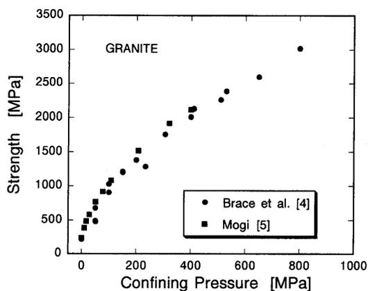
Fig.1. Compressive fracture strength of Westerly granite.
