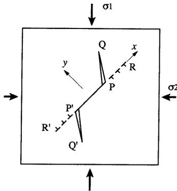
Fig.10. Sliding crack model with plastic zones PR and P'R'. From Horii and Nemat-Nasser [68].
