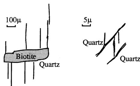
Fig.7. Sketch of stress-induced cracks. Max. compressive direction is vertical direction, and confining pressure is horizontal direction. After Tapponnier and Brace [31].
