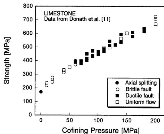
Fig.2. Compressive fracture strength of limestone with macroscopic failure mode, Failure mode changes from Axial splitting to Brittle fault, to Ductile fault, and to Uniform flow.
