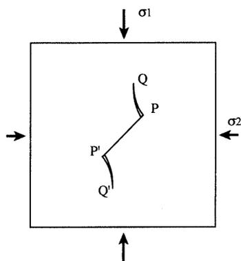
Fig. 8. Sliding crack model: model of flaw under compression; PP': Initial angled crack; PQ and P'Q': Tension crack.
