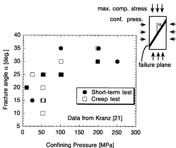
Fig.6. Fracture angle  $\alpha$  of Barre granite in creep tests and short-term tests. Fracture angle is defined as the angle from the direction of the maximum compressive stress to the failure plane direction.
