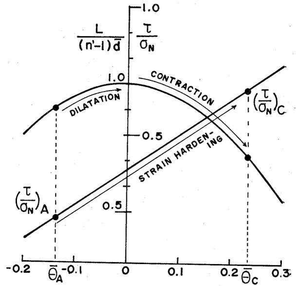
Fig. 13. Change of  $\bar{\theta}$  mobilized stress ratio and length  $L$  given by Eq. (16) during the strain hardening process up to the peak stress ratio  $(\tau/\sigma_N)_C$
