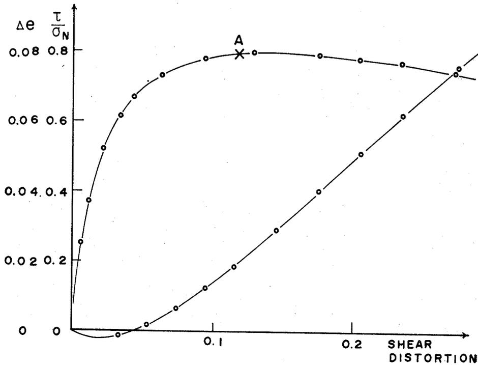
Fig. 14. Typical curves showing relations between stress ratio, shear distortion and change of void ratio in simple shear test of granular soil (Cole, 1967)
