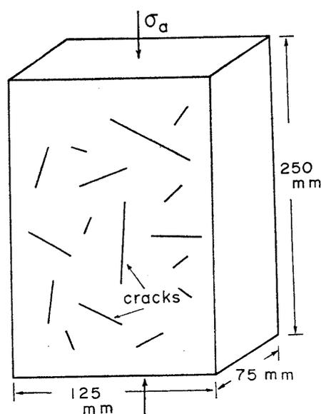
Fig. 6. Gypsum plaster sample with random cracks
