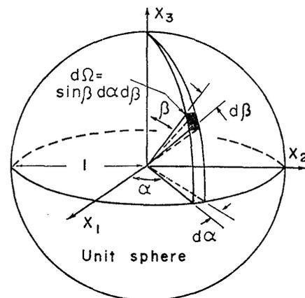
Fig. 1. Unit sphere to define solid angle  $d\Omega$
