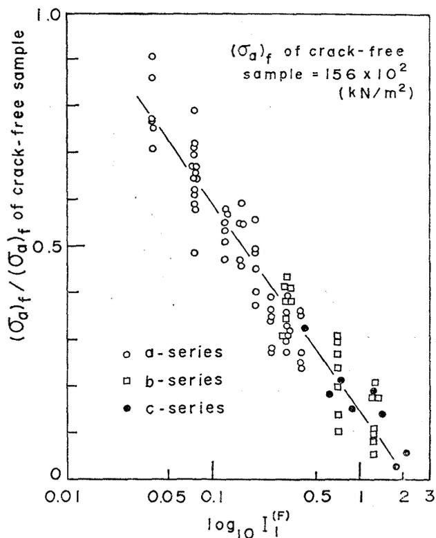
Fig. 8. Linear relation of uniaxial compressive strength  $(\sigma_a)_f$  to logarithm of first invariant of  $F_{ij}^{(R)}$
