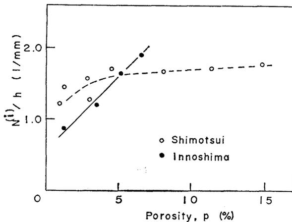
Fig. 11. Number of cracks crossed by unit length of  $i$ -scanning line
