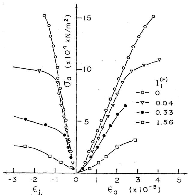
Fig. 7. Relation between axial stress  $\sigma_a$ , axial strain  $\epsilon_a$  and lateral strain  $\epsilon_l$  for four gypsum plaster samples having different values of first invariant of  $F_{ij}^{(R)}$
