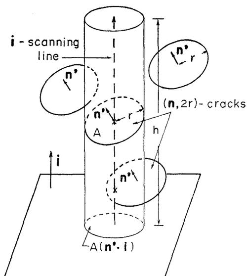
Fig. 2. A column of volume  $Ah(\mathbf{n}' \cdot \mathbf{i})$  whose center line accords with  $\mathbf{i}$ -scanning line (Note that if the centers of  $(\mathbf{n}', 2r)$ -cracks are located inside the column, these must cross the  $\mathbf{i}$ -scanning line)
