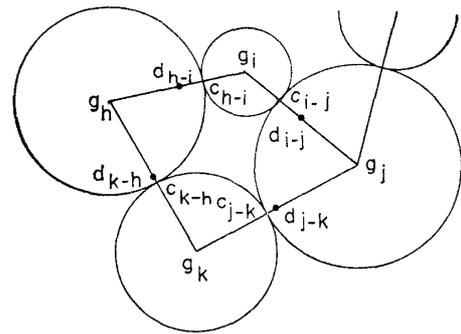
**Fig. 3.** An assembly of spheres replaced by an assembly of lines (called branches) connecting centers of adjacent particles which are in contact at points ( $g_i$ =center of sphere;  $c_{i-j}$ =contact between spheres  $g_i$  and  $g_j$ ;  $d_{i-j}$ =mid-point of branch  $\overline{g_i g_j}$ )
