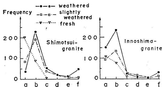
Fig. 10. Progressive change of cracks due to weathering of granite (Onodera, Yoshinaka and Oda, 1974)
