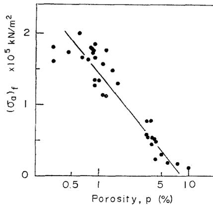
Fig. 12. Relation between uniaxial compressive strength  $(\sigma_a)_f$  and porosity  $p$  of granite (modified from Yoshinaka's (1973) data) (Note that this linear relation is quite similar to the relation of Fig. 8)
