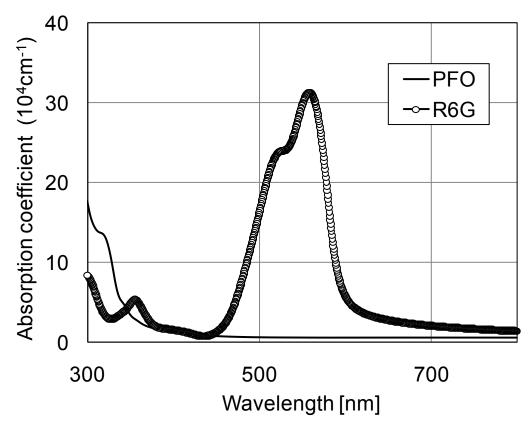
Fig. 1 Absorption spectra of R6G and PFO neat films.
