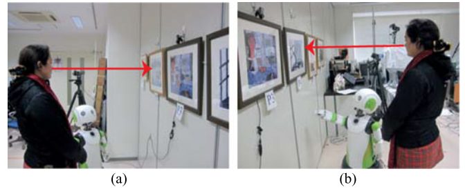
Fig. 7. Robot's position for interaction: (a) Robot selects the left-side interaction path when the visitor's orientation of attention is detected in the LNPFV area. (b) Robot selects the right-side interaction path when the visitor's orientation of attention is detected in the RNPFV area.
