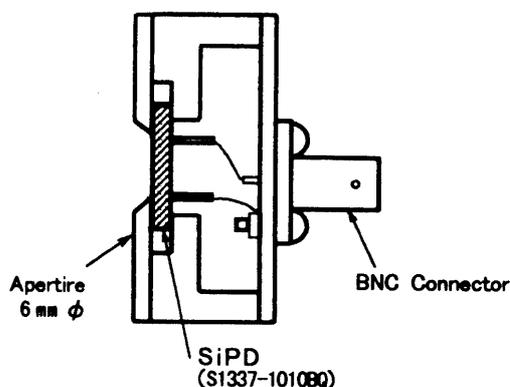
Fig.6 Construction of spectral responsivity transfer photodiode compared with participants' standard.
