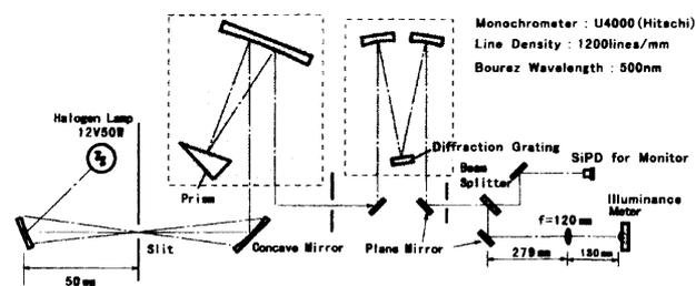
Fig.2 Configuration of the participant A and D's spectral responsivity measurement.
