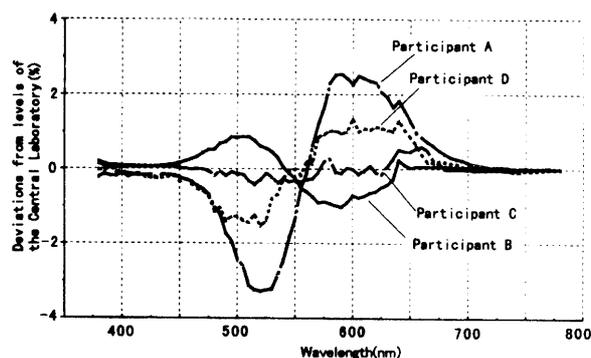
Fig. 8 Percent differences from center lab of all participants' spectral responsivity measurements for transfer illuminance meter.
