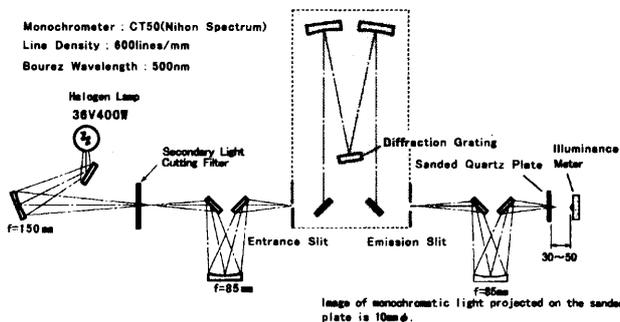
Fig.3 Configuration of the participant B's spectral responsivity measurement system.
