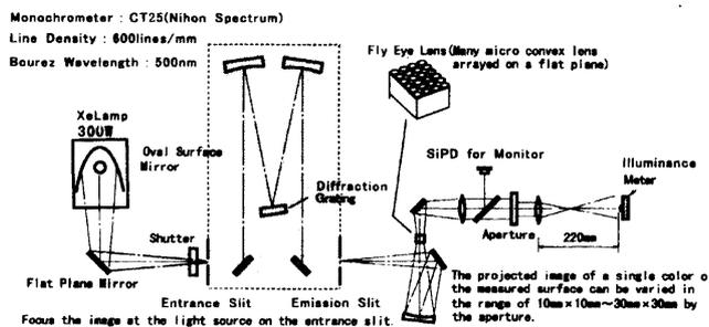
Fig.4 Configuration of the participant C's spectral responsivity measurement system.
