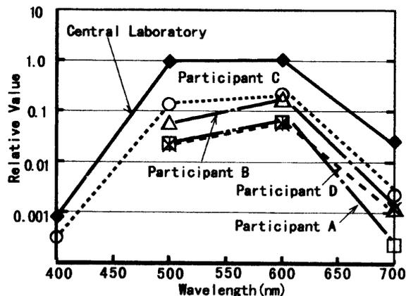
Fig.5 Output of participants' spectral responsivity measurement systems for transfer illuminance meter.
