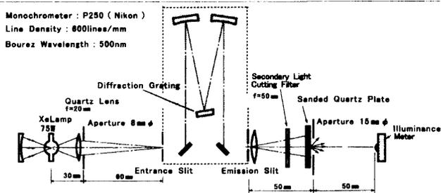
Fig.1 Configuration of the center lab's spectral responsivity measurement system.
