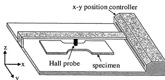
Fig. 2. Experimental setup for leakage magnetic flux measurement.
