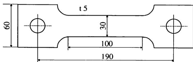
Fig. 1. Specimen configuration.
