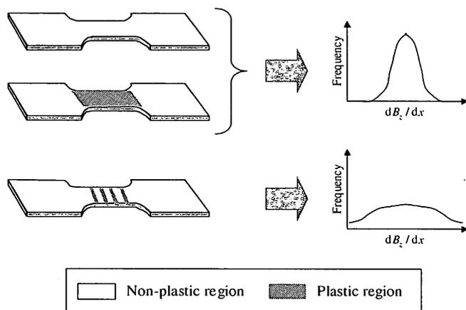
Fig. 15. Schematic illustration showing that the full width at half maximum (FWHM) for the frequency distribution profile of the  $dB_z/dx$  increases when both plastic and non-plastic region existed on the plate-type specimen.
