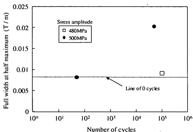
Fig. 14. Change in the full width at half maximum (FWHM) with stress cycling for the fatigued specimens.
