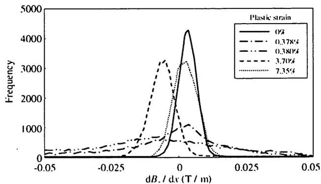
Fig. 11. Frequency distribution of the  $dB_z/dx$  for the tensile specimens.
