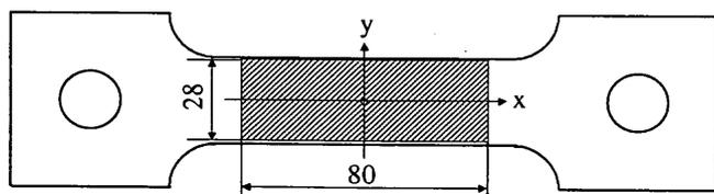
Fig. 3. Scanning area of leakage magnetic flux.
