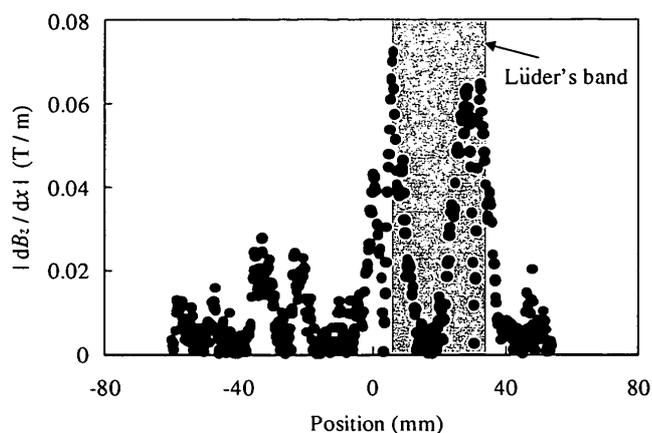
Fig. 6.  $|dB_z/dx|$  distribution with 0.378% plastic strain on the line of  $y=0$ .
