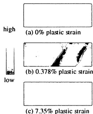
Fig. 9. Change in the pattern of the  $dB_z/dx$  distribution with plastic strain for the tensile specimens.
