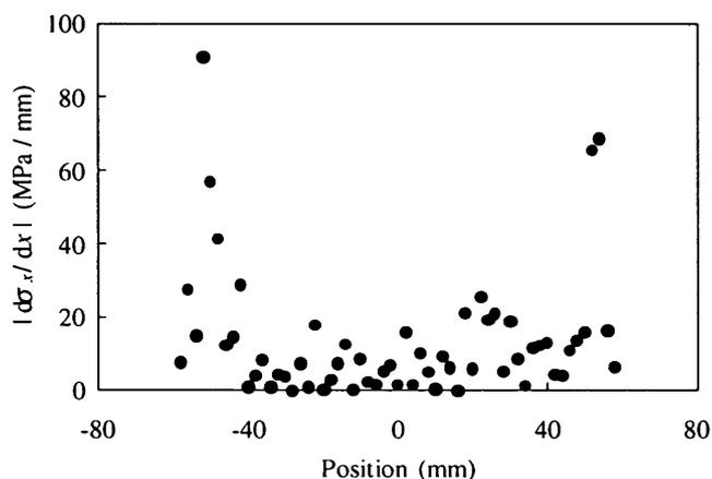
Fig. 7.  $|d\sigma_x/dx|$  distribution with 7.35% plastic strain on the line of  $y=0$ .
