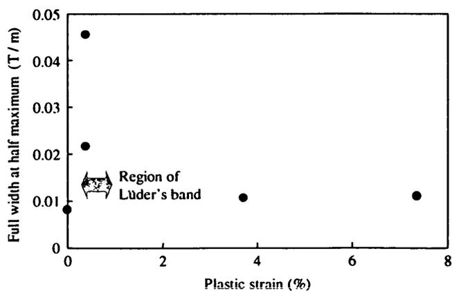
Fig. 13. Relationship between the full width at half maximum (FWHM) and applied plastic strain for the tensile specimens.
