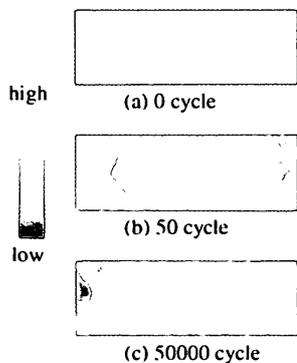
Fig. 10. Change in the pattern of the  $dB_z/dx$  distribution with stress cycling under stress amplitude of 500MPa for the fatigued specimens.
