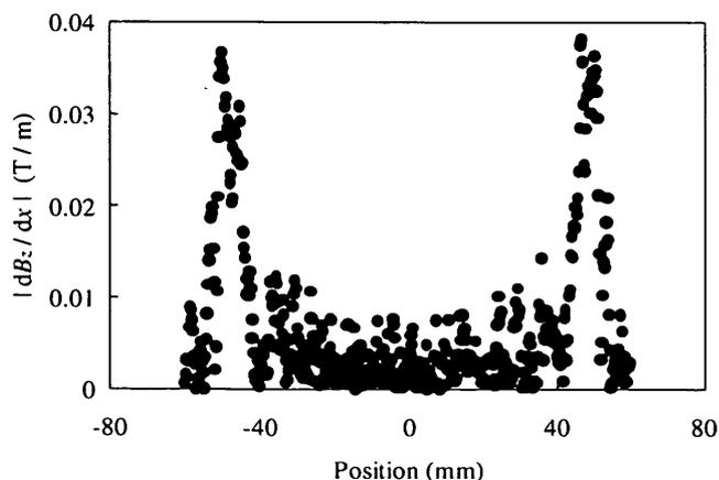
Fig. 5.  $|dB_z/dx|$  distribution with 7.35% plastic strain on the line of  $y=0$ .
