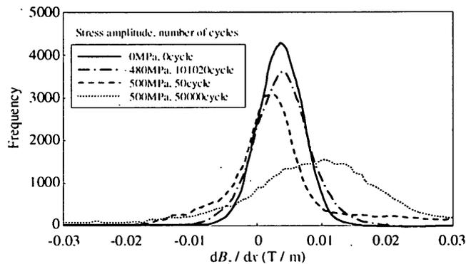
Fig. 12. Frequency distribution of the  $dB_z/dx$  for the fatigued specimens.
