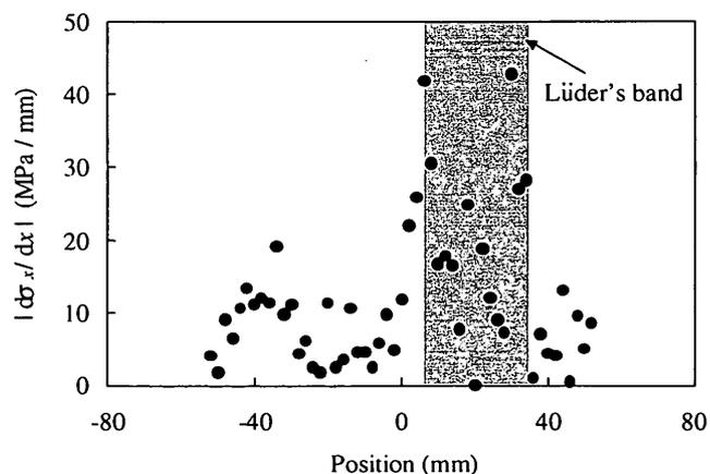
Fig. 8.  $|d\sigma_x/dx|$  distribution with 0.378% plastic strain on the line of  $y=0$ .
