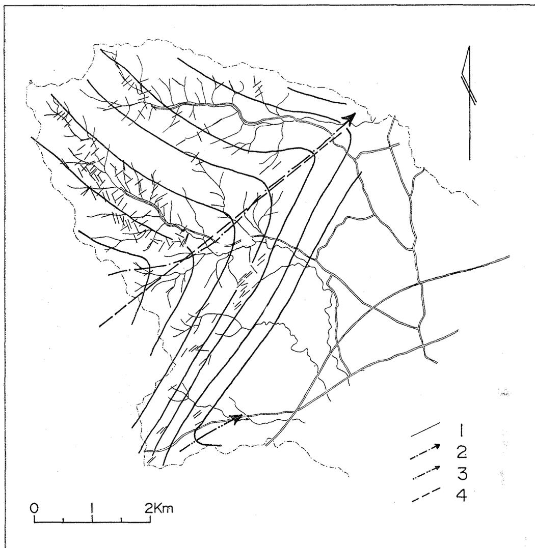
Fig 2. Folded screen structure of Miocene pyroclastic formation in Oyama-Isehara district, central Japan.
