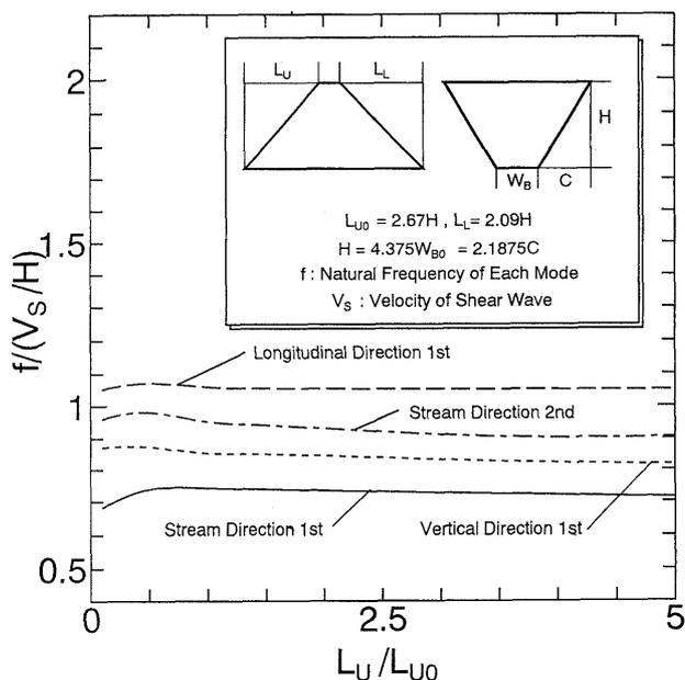
**Fig. 15. Variation of dimensionless eigenfrequencies up to lower 4th order modes according to the change in dam slope of up stream side**
