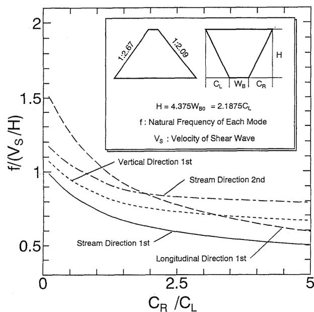
**Fig. 16. Variation of dimensionless eigenfrequencies up to lower 4th order modes according to the change in dam slope of right abutment only**
