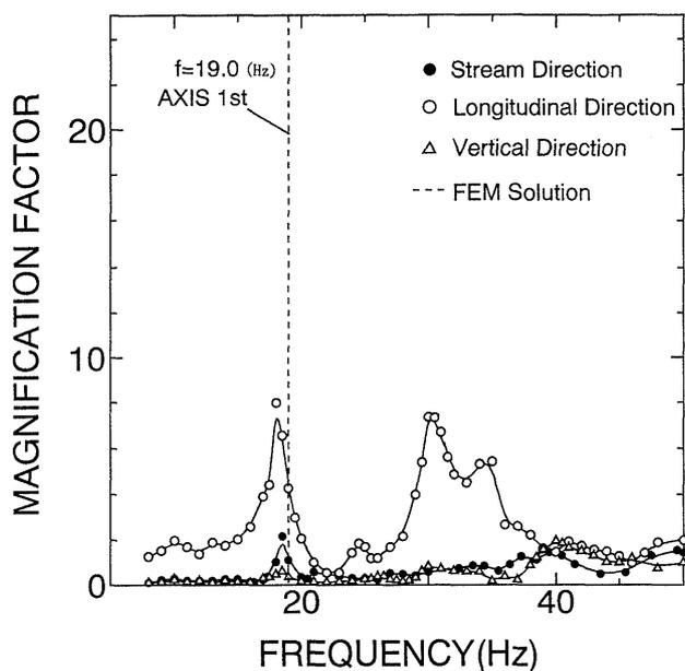
Fig. 9. Resonance curves at  $2H/3$  point on dam slope (for the case of excitation in longitudinal direction)
