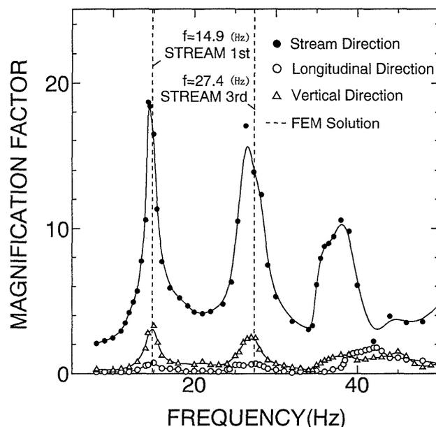
**Fig. 3. Resonance curves at center on dam crest (for the case of excitation in stream direction)**
