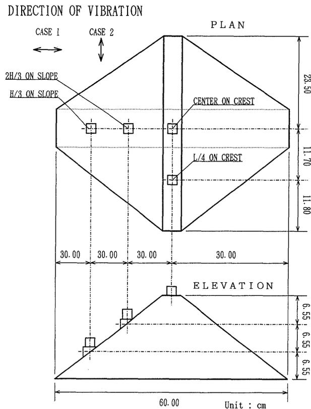
**Fig. 2. Arrangement and positions of accelerometers**
