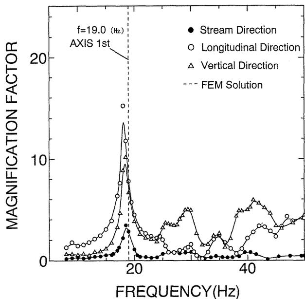
Fig. 8. Resonance curves at  $L/4$  point on dam crest (for the case of excitation in longitudinal direction)
