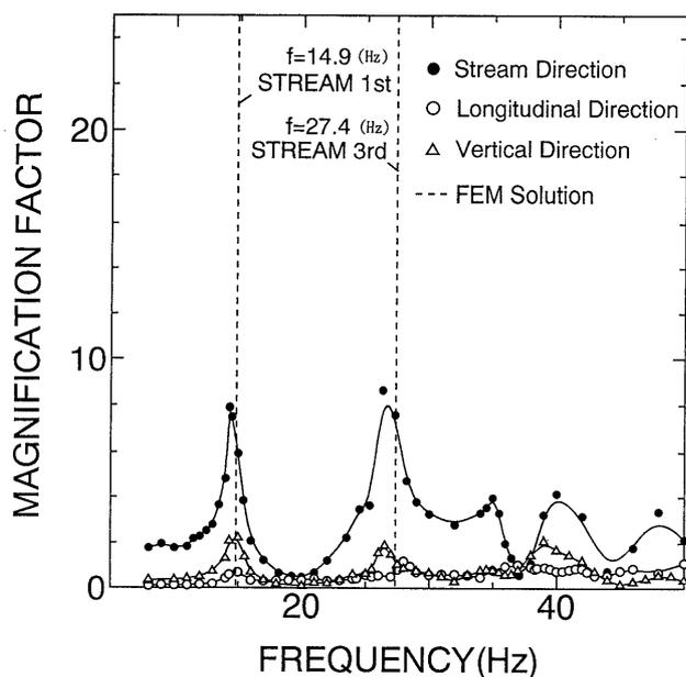
Fig. 4. Resonance curves at  $L/4$  point on dam crest (for the case of excitation in stream direction)
