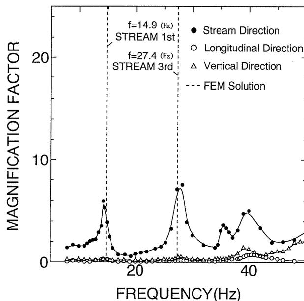
Fig. 6. Resonance curves at  $H/3$  point on dam slope (for the case of excitation in stream direction)
