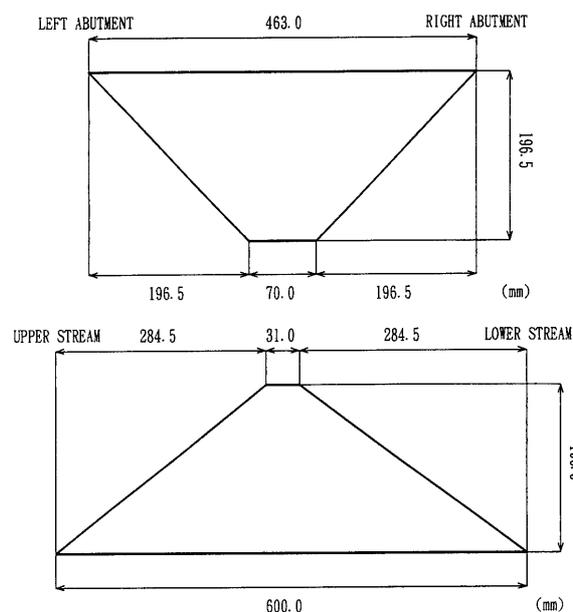
Fig. 1. Vertical cross sectional views at center on dam crest
