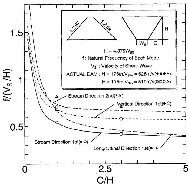
Fig. 18. Variation of dimensionless eigenfrequencies up to lower 4th order modes according to the change in both slopes of symmetry abutments
