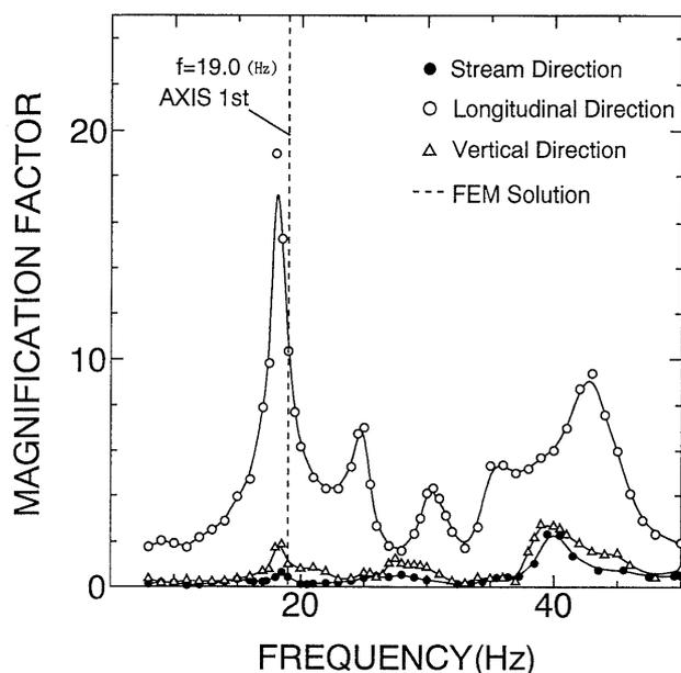
Fig. 7. Resonance curves at center of dam crest (for the case of excitation in longitudinal direction)
