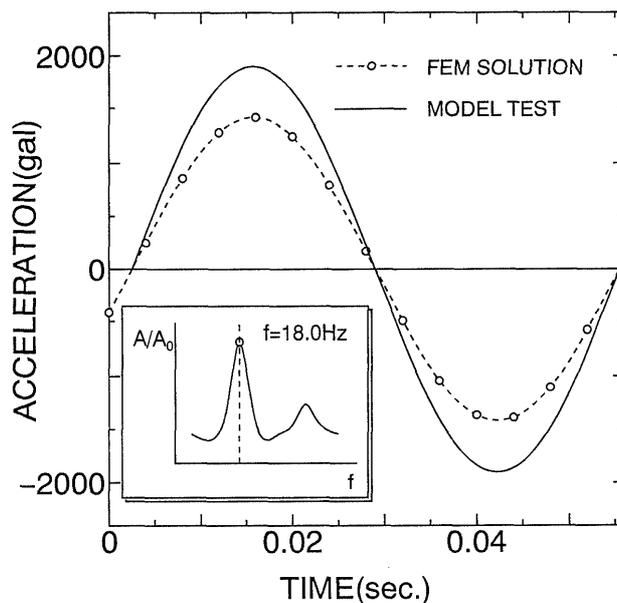
Fig. 14. Time history of acceleration in steady states for the 1st mode in longitudinal direction (Experimental and numerical results)
