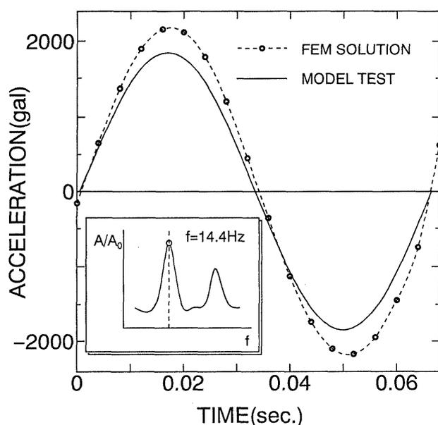
Fig. 13. Time history of acceleration in steady states for the 1st mode in stream direction (Experimental and numerical results)
