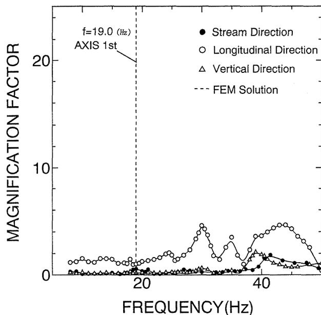
Fig. 10. Resonance curves at  $H/3$  point on dam slope (for the case of excitation in longitudinal direction)
