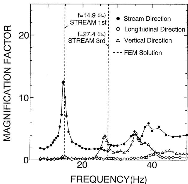
Fig. 5. Resonance curves at  $2H/3$  point on dam slope (for the case of excitation in stream direction)
