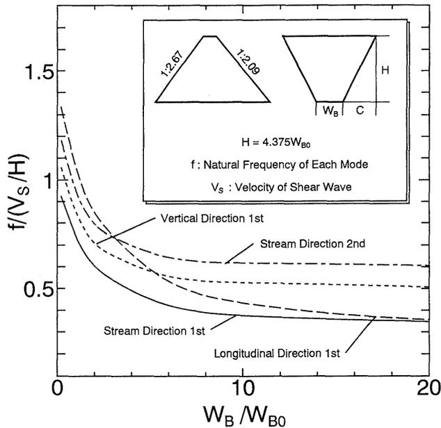
Fig. 17. Variation of dimensionless eigenfrequencies up to lower 4th order modes according to the change in width of riverbed
