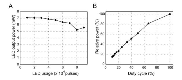
Figure 2. Assessment of battery life and adjustability of blue LED power. (A) Black circles indicate the averaged output powers of the LED after multiple 10,000 pulses of 25 ms duration. The output power remains relatively stable for the first 30,000 pulses. (B) Each black circle indicates the relative average LED power modulated by the frequency of 400 µs pulses within 300 ms. The output power linearly increases with the duty cycle.
