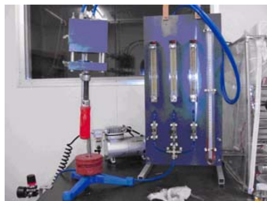
Fig. 2 Setup for the measurement of air permeability.
