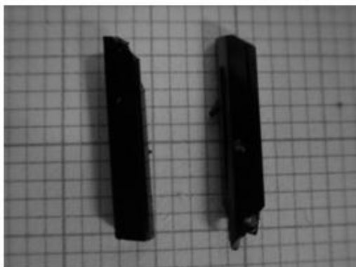
Fig. 1 World-record size crystals of charge transfer complex \beta' -(BEDT-TTF) 2 ICl 2 (c. 50mg).
