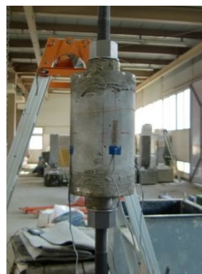
Fig.3 Direct tension test
