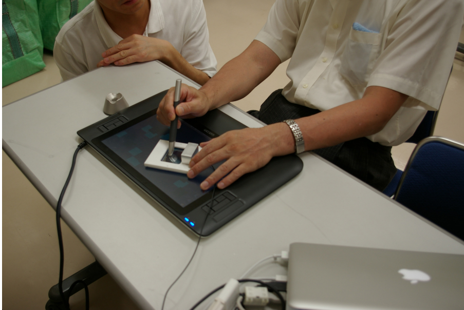
Fig. 5.11 Demonstration of pen tablet type SAW tactile display for blind persons
