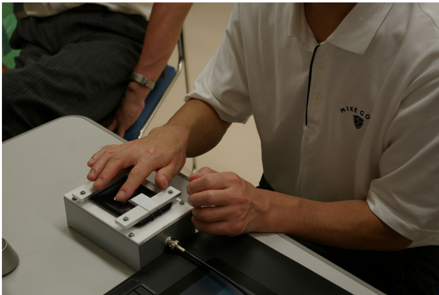
Fig. 5.12 Demonstration of tactile display using sheet-type ultrasonic transducer for blind persons
