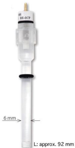
Figure 3.3. A picture of the Ag/AgCl reference electrode. ( https://www.als-japan.com/1388.html )
