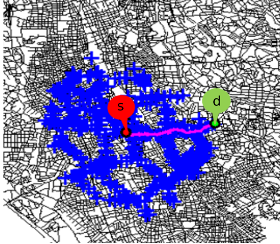
Figure 2.7: The example of shortest path searching between s and d on road map and the way of expansion of the searching area in the SPFMM approach.
