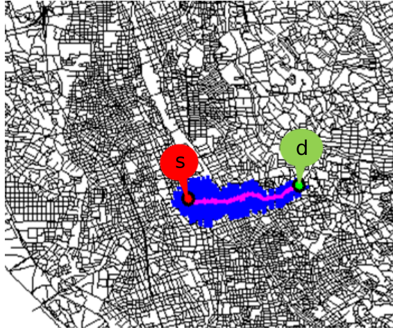
Figure 2.5: The example of shortest path searching between s and d on road map and the way of expansion of the searching area in A^* algorithm.
