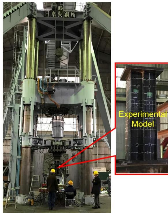
Fig. 4.13 Test setup in the fatigue testing machine with a static load capacity of 6,000kN.
