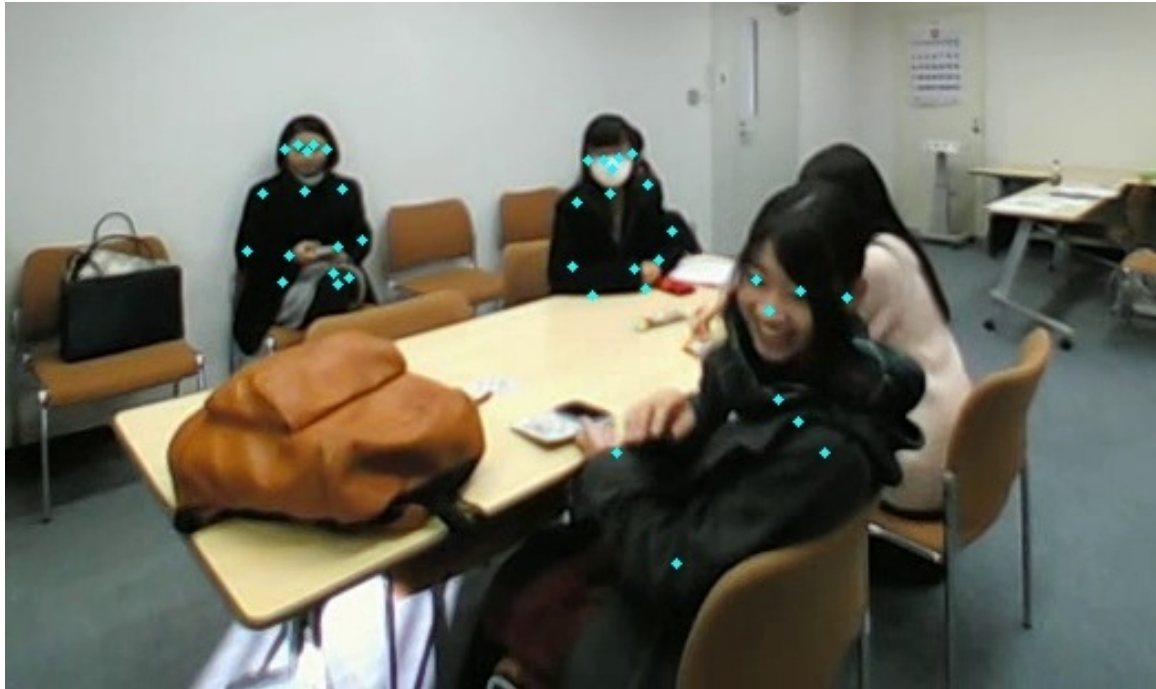
Figure 3.3: Example of Key-point of Individual Person in the Scene using USB Web-camera
